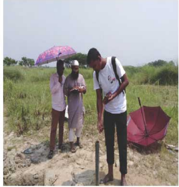
Figure-6: Measurement of Ground Water level
