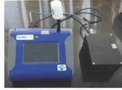
Dust Trak Aerosol Monitor
